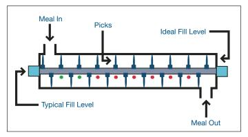
Increasing the fill level provides greater distribution of steam through the meal as will feeding the steam into the conditioner below the meal.
