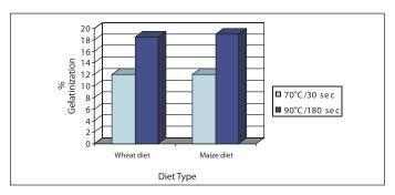
Figure 5 clearly shows that increased conditioning time and temperature increases gelatinization in feed, regardless of the cereal base used. The process of gelatinization creates natural 'glues' which allows the feed particles to compress tightly and adhere to each other when passing through the pellet die. Optimal 'cooking' of feed will result in more durable pellets and reduce levels of fines (Figure 6).
