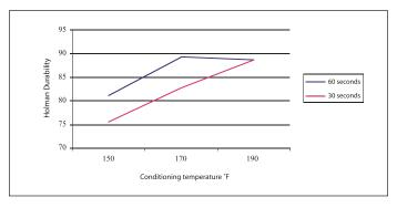
As the conditioning time and temperature was increased, the pellet durability increased (as expressed by a Holmen Durability Index).
