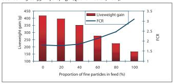
The majority of commercial broiler diets have been through the pelleting process. However, the durability of pellets can be variable, resulting in levels of fines as high as 50%. Incidences of high levels of fines in the field are associated with poor liveweight and FCR. To maximize performance, the accumulation of fine particles in the feed should be minimized.
