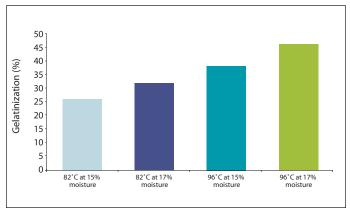
Some feed additives can also improve the conditioning process; new moisture and surfactant technologies allow the addition of moisture at the mixer or conditioning chamber which can greatly improve feed pellet quality. The addition of the moisture and the improved pellet quality has
